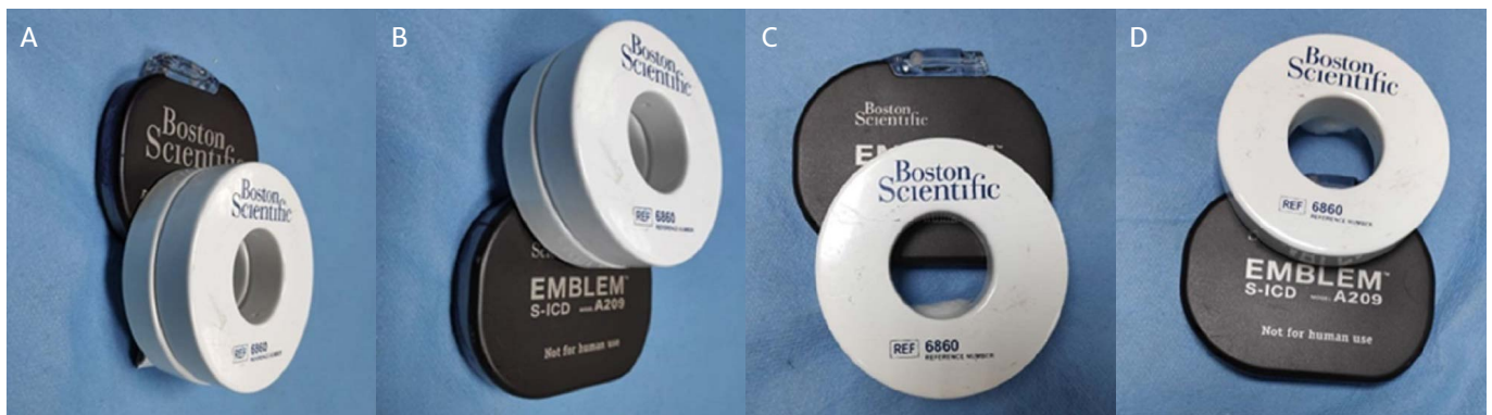
FIGURE 3. Correct position of double magnets and specific donut magnet position. A – Double magnet application in obese patients with Emblem S-ICD A209 – the magnet should be applied on the upper edge; B – Double magnet application in obese patients with Emblem S-ICD A219 – the magnet should be applied on the lower edge; C – Emblem S-ICD A209 – the magnet should be applied on the upper edge; D – Emblem S-ICD A219 – the magnet should be applied on the lower edge
