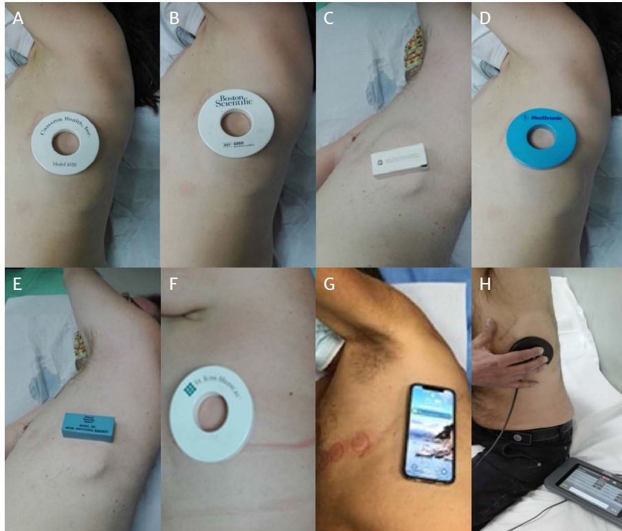
FIGURE 1. The tested magnet in vivo with the 4520 Boston Scientific model (A), the 6860 Boston Scientific model (B), the Biotronik model (C), the Medtronic model (D), the LivaNova (formerly ELA/Sorin) model (E), the Abbott (formerly St. Jude Medical) model (F), the iPhone 12 Pro Max (G); the interrogation of the S-ICD device with the Model 3200 programmer (H)
